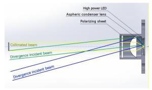
Figure 2: Lighting modules and beam divergence.
