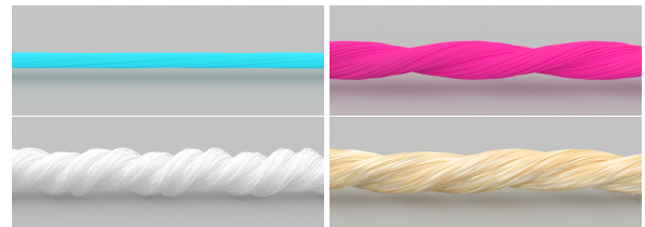
Figure 11: Renders of virtual replicas of the Gütermann sewing yarns described in Table 3. From left to right, and top to bottom, the yarns are Skala360 (polyester), ORA 120 (polyester), CNe 50 (cotton), and S 303 (silk), with varying DoS.
